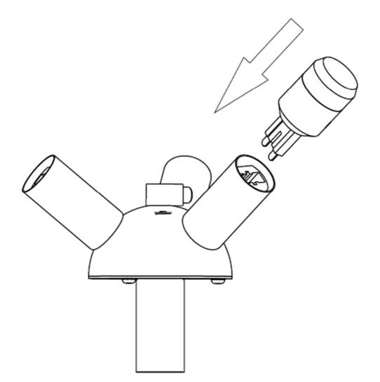
Replacement of the light source should be provided by qualified technician to prevent any damage to health or property.
