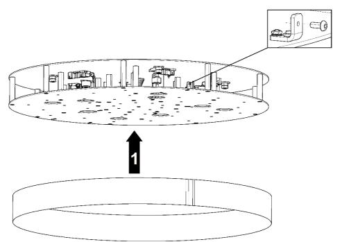
5. Install outside side polished stainless steel cover plate to the bearing frame as shown on sketch below, foil covered side should be facing outside, foil should be removed after installation of frame to fixing points.
