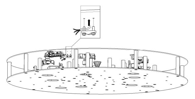
3. Fix the power cable to the top bearing plate by cable clamp(as shown above).
